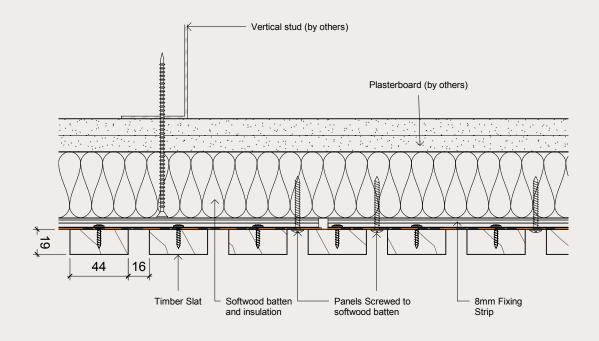
STOCK panels can be used for both horizontal AND vertical internal walls and can use a variety of fixing methods.
